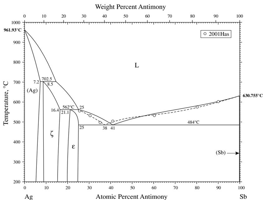
**Fig. 1** Ag-Sb Phase Diagram
